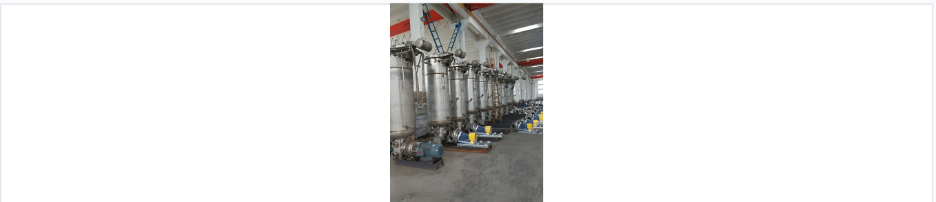
Stainless steel dyeing vessels with integrated pumps and automation systems.
