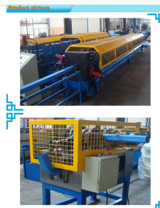
High-capacity roll forming system for downpipe production.
