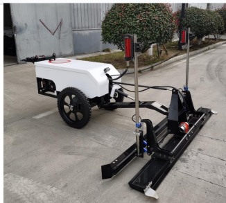
A precise leveling process driven by an integrated hydraulic head.
