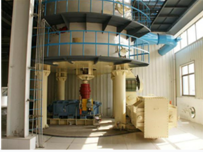
Robust desolventizer unit with heavy-duty support columns.
