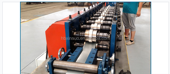
High-precision rollers designed for consistent shaping of building profiles.
