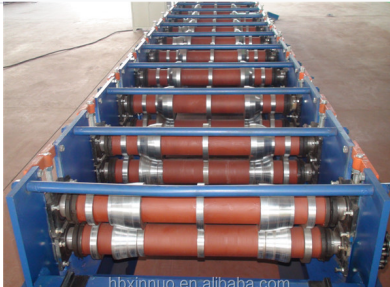
Gradual metal shaping through multiple roller passes
