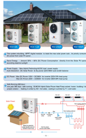
System architecture showing solar PV integration, MPPT control, and city power balancing.
