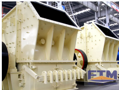
A detailed view of the single-stage crusher, highlighting its heavy-duty construction designed for primary crushing in mining operations.
