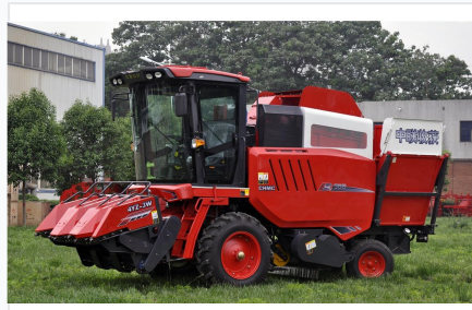
Advanced 4-row harvesting head designed for efficient crop gathering.
