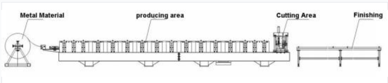
Workflow overview showing material feeding, forming, and automated cutting stations.
