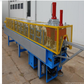
Main roll forming assembly showcasing the robust frame and drive system.
