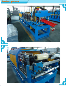
Precision forming stations for consistent ridge cap quality.
