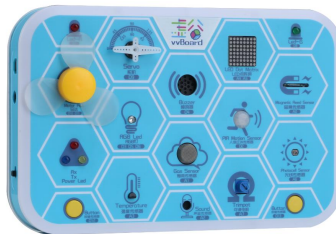
Integrated experiment box featuring various sensors and output modules for hands-on programming education.
