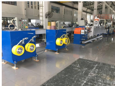
Full view of the PP strapping production line featuring stainless steel tanks and PLC interface.
