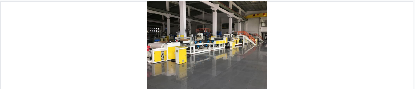
Full view of the 1000mm PP ribbon film extrusion production line featuring integrated stretching and winding units.
