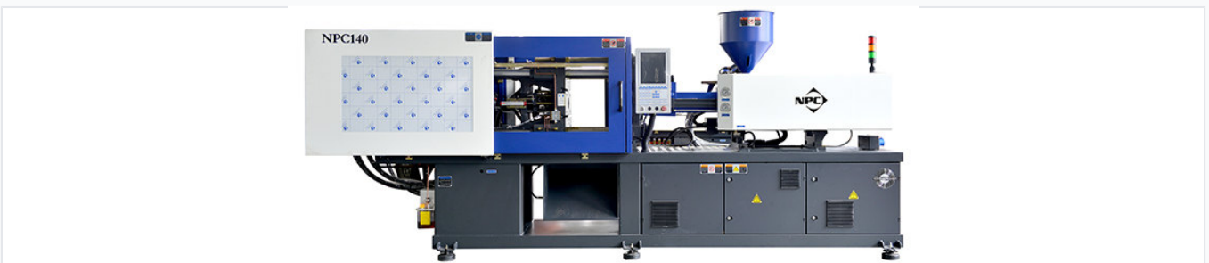
Overview of the high-performance NPC 140 molding machine.
