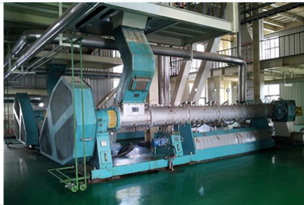
Extruder system for mechanical oil processing.
