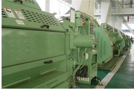
Flaking mill unit designed for uniform flake thickness.
