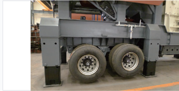
Mobile unit with hydraulic support legs for stability during operation.
