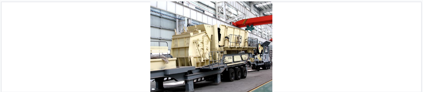
A robust mobile concrete crusher mounted on a heavy-duty trailer, featuring a large hopper and discharge conveyor for efficient on-site material processing.
