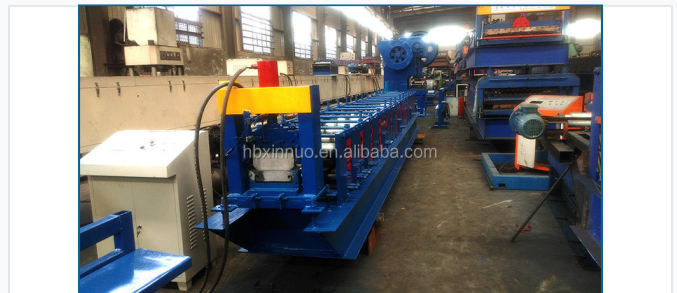
Versatile machine combining roof tile making, metal sheet shearing, and roll forming.
