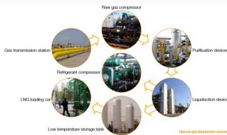
A detailed layout of the natural gas liquefaction process, highlighting the flow from transmission to final loading.
