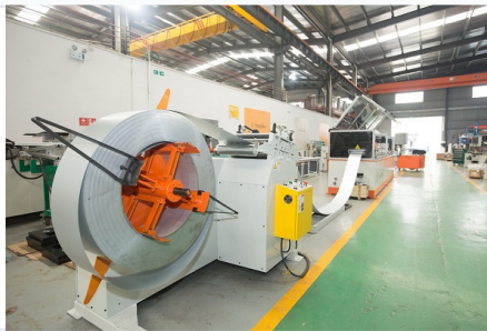
The machine features an automatic uncoiler and multi-stage roll forming process for consistent quality.
