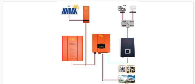
System integration diagram showing compatibility with solar, utility, and generator power sources.
