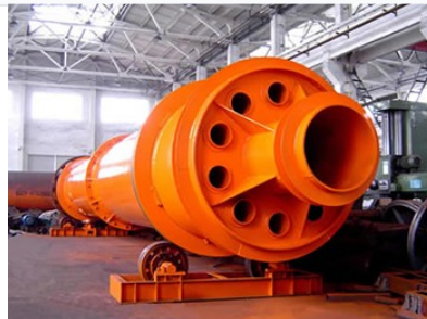
A robust industrial rotary dryer designed for efficient indirect heat transfer in mining and construction applications.
