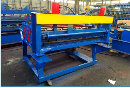
Detailed view of the hydraulic system, rollers, and adjustable blades.
