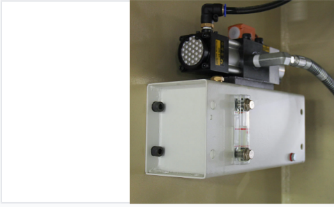
Detail view of the hydraulic reservoir, liquid level indicator, and pneumatic filtration system for precise control.
