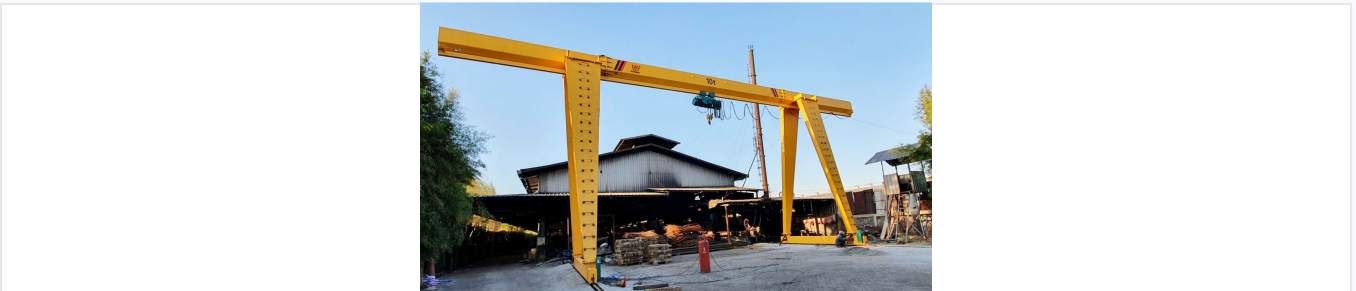
10-ton capacity single girder gantry crane designed for outdoor material handling.
