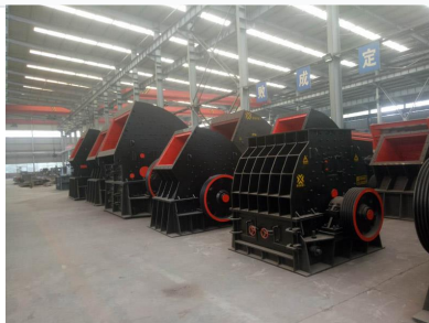
The heavy-duty hammer crusher engineered for primary and secondary crushing.
