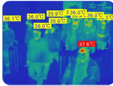
Software interface featuring automatic tracking and alarm triggers for elevated temperatures.
