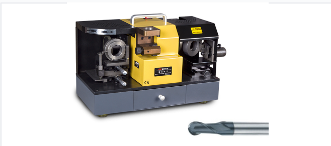
Specialized grinder for precision sharpening of ball end mills.
