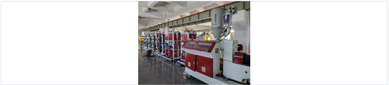
Full view of the automated carrier tape production line featuring extrusion and forming stations.
