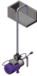
Detailed view of the flow switch integrated into a pump and pressure tank assembly.
