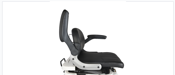
Ergonomic seat designed for rider comfort with adjustable backrest.
