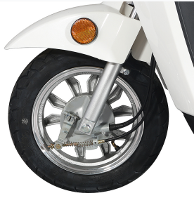
Front wheel assembly featuring tubeless tire and drum brake system.
