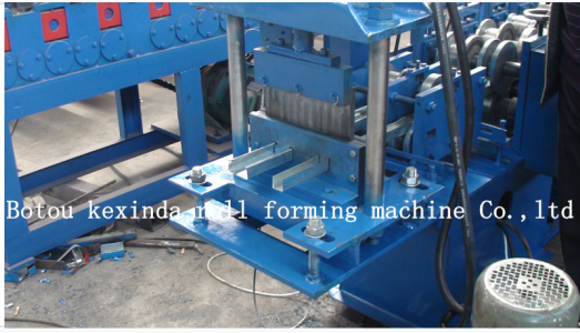
Robust frame construction with integrated cutting mechanism for length control.
