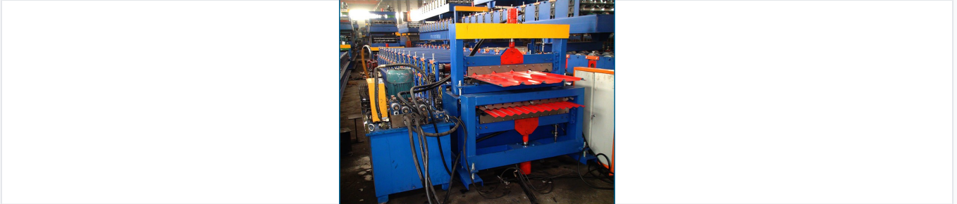
Heavy-duty blue and yellow frame construction showing the roller series for dual-profile production.
