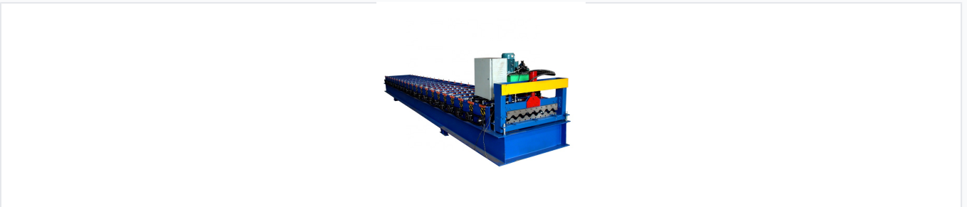
The complete roll forming line featuring a multi-stage forming section and integrated control system.
