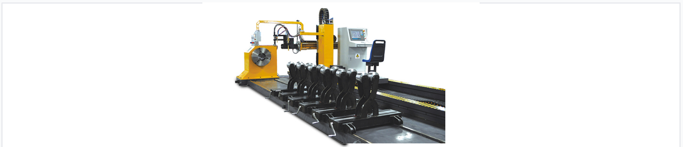
The robust gantry system and rotary chuck allow for high-precision processing of various pipe lengths.
