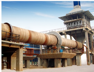
A robust cement kiln designed for efficient heat transfer and material processing in large-scale manufacturing.
