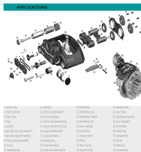
Detailed technical diagram showing the internal assembly and components of the brake caliper.
