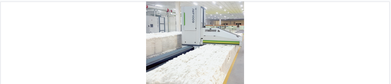
Primary view of the JWF1009 bale plucker in a standard blow room configuration.
