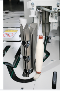
Precision metal guides ensure accurate yarn placement during high-speed winding operations.
