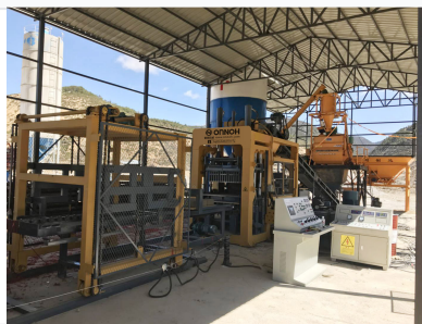
The main engine unit features high-strength welded construction and integrated hydraulic controls.
