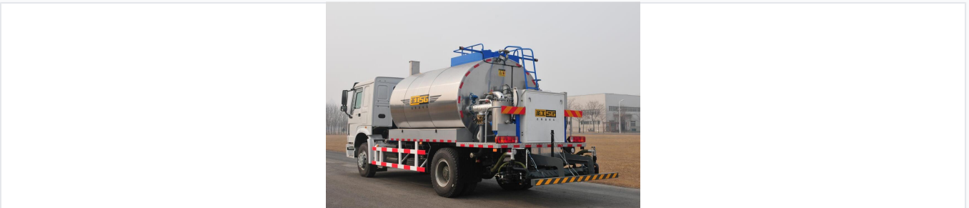
Fully equipped asphalt distributor truck ready for road maintenance duties.
