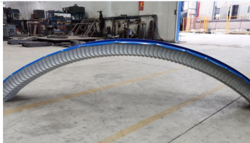
The machine produces high-precision curved panels for self-supporting structures.
