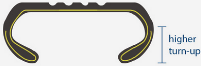
Reinforced high reversed carcass structure
