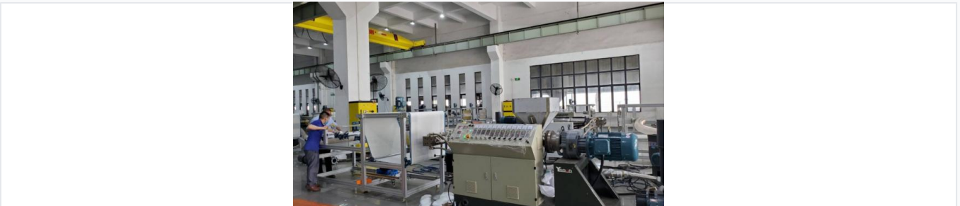
The complete AF-600mm production line integrating extrusion, air-blowing, and web-forming technologies.
