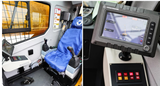
Advanced control console with load monitoring display.
