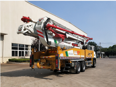
Multi-section boom system extended for maximum reach.
