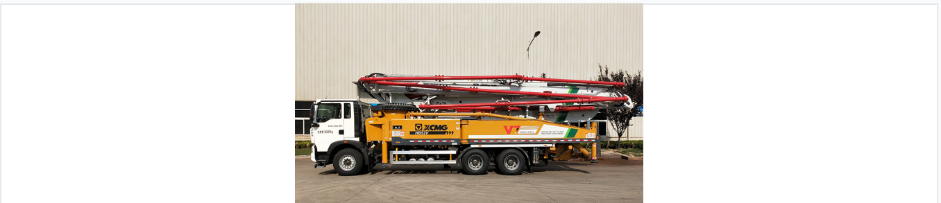
Side view of the 52-meter boom concrete pump truck.
