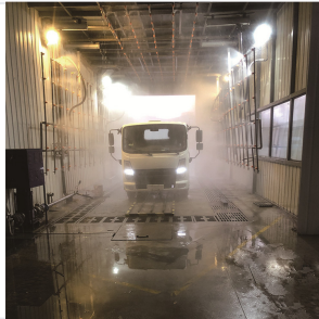
Pre-delivery rain and wash testing to verify cabin sealing and electrical protection.
