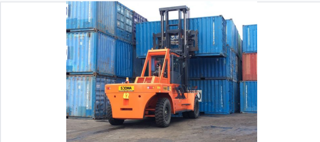
A robust 30-ton diesel forklift designed for high-capacity industrial lifting.
